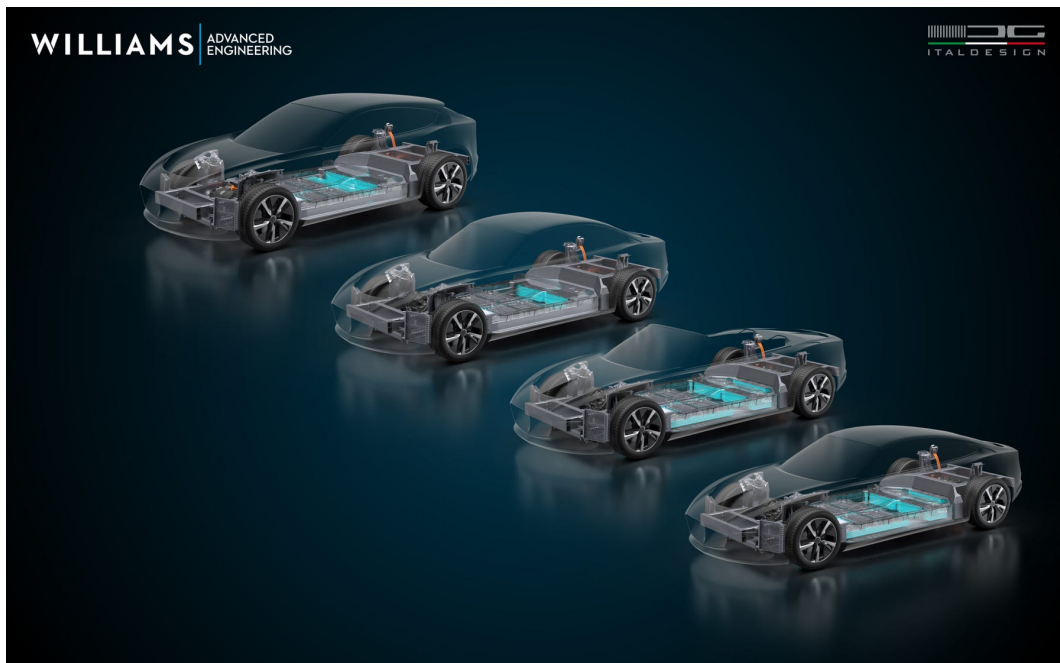
Figure 1: Williams Advanced Engineering (WAE) and Italdesign are cooperating on a modular platform for building a wide variety of high-end electric cars.
