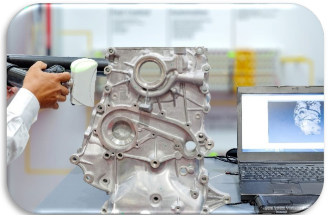
Figure 3: 3D scanner in the process of scanning.
