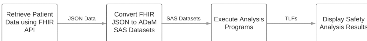
Figure 1. High-level Process Diagram for Safety Analysis using CDISC ADaM and HL7 FHIR
