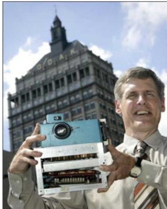
Steven Sasson holds the prototype digital camera he built in 1975 at the Eastman Kodak Co. headquarters in Rochester, N.Y. It recorded a black-and-white image on a digital cassette tape. Photo: /Associated Press / AP
